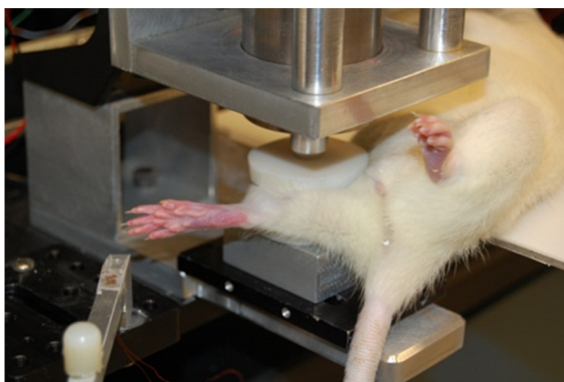
Fig. 2 Table setup version of a knee-loading device used for testing the knee of a rat
